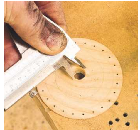
▲ Pic.24 He needs to tie the little flat on the top with the base of the finial. The measurement will be transferred to the stem with the Vernier callipers
